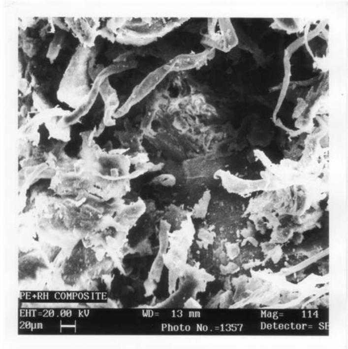
Figure 3 SEM micrograph I of paper sludge composite
